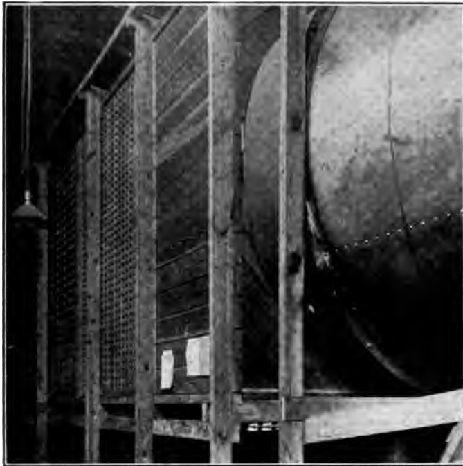
FIG. 7. EXTERIOR OF THE WIND TUNNEL AT THE MASSACHUSETTS INSTITUTE OF TECHNOLOGY, SHOWING CELLS THROUGH WHICH AIR IS SUCKED IN FROM THE ROOM
